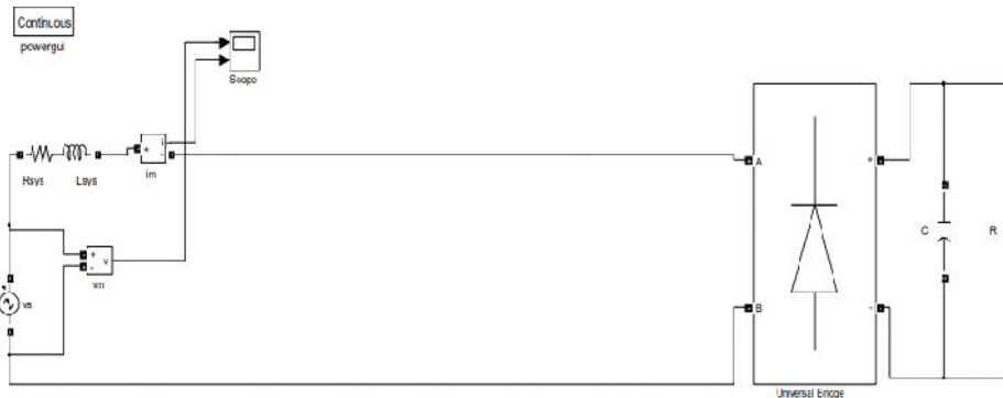
Fig 15: Simulation of equivalent SM.
