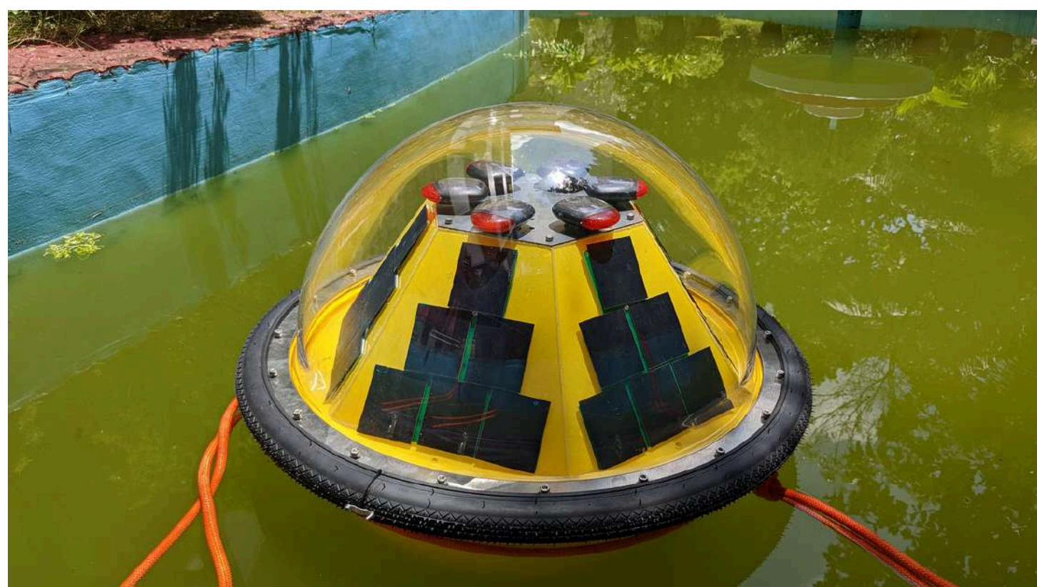
Fig.14.3.42. Buoy developed by CUSAT to monitor marine habitats
