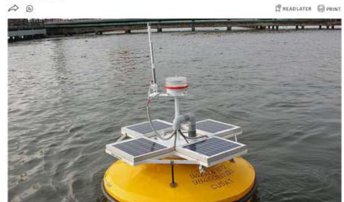
Fig.14.3.40. The launched ocean data buoy system by the Department of Physical Oceanography, CUSAT
